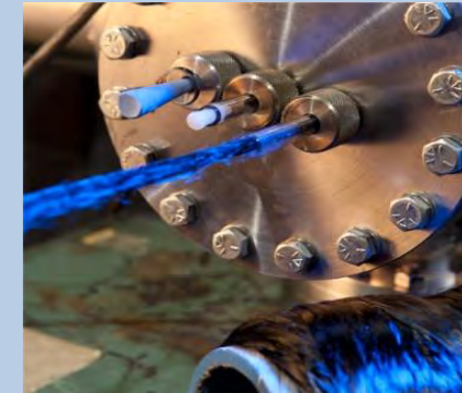
Exit end of Microwave Assisted Plasma (MAP) process, jointly developed by ORNL and Dow
