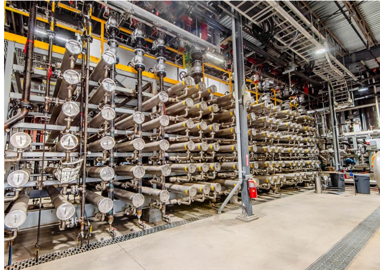
Black Liquor Membrane Separation System at IP's Grande Prairie Mill in Alberta, Canada. Image Credit: Via Separations
